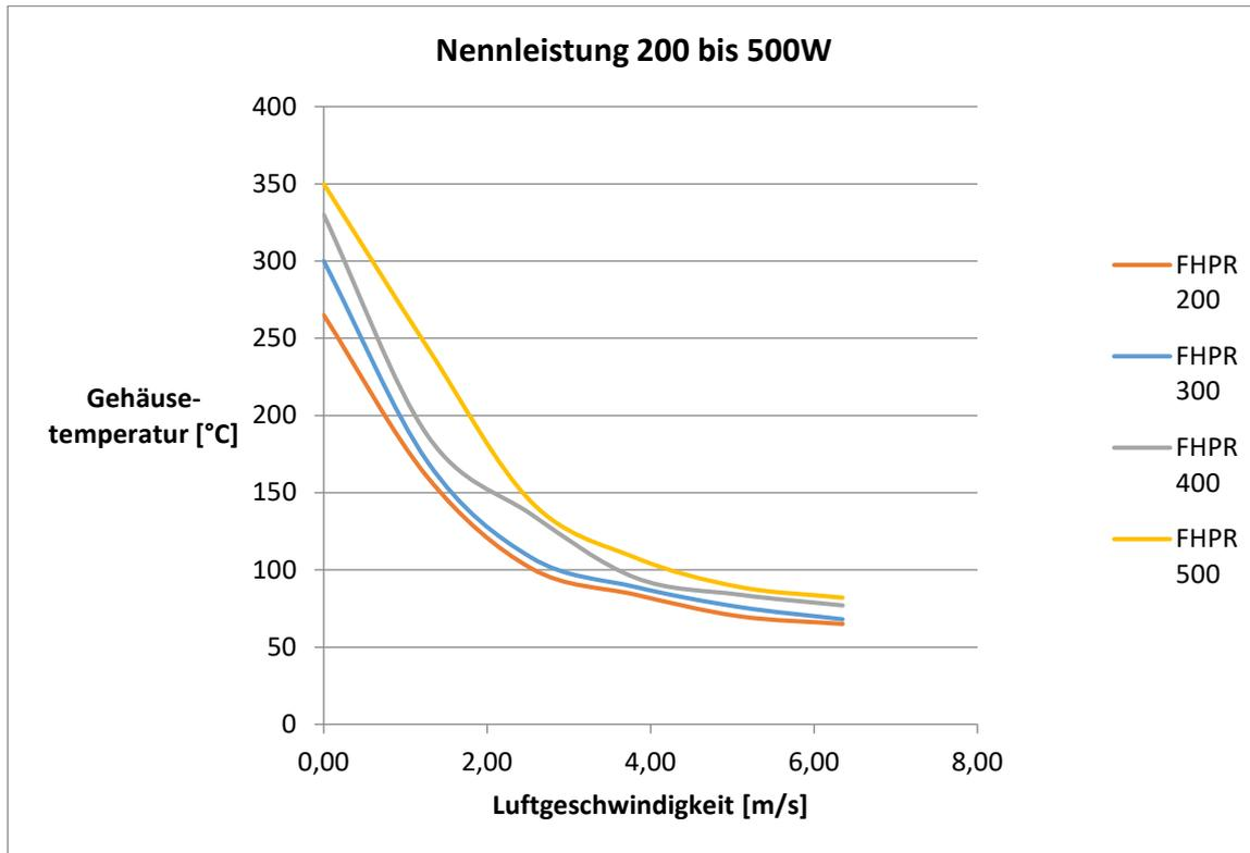
**Surface temperature rate depending on air speeds**
